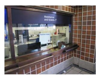
Edmonds specialise in the setting out, manufacture and installation of bespoke tube & station ticket offices. We carried out the initial prototype at Kings Cross inconjunction with Arup and have since completed numerous other stations to to same detail although have incorporated design improvements. The contracts included formation of stainless steel or bronze frontages, ballistic cash boxes, trespa & ergonomic counters and backfittings.
